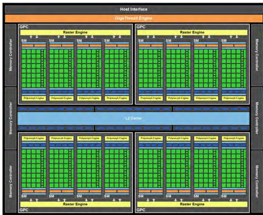
The GF100 architecture in detail
